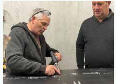
Paul Harris demonstrates a new laser welder that will take care of thin wall 5mm to 0.5mm, high precision jobs
